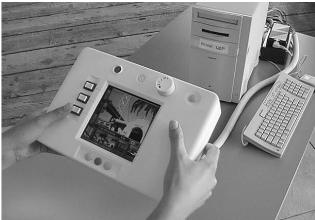
Figure 6: Digital camera interaction architecture prototype.
